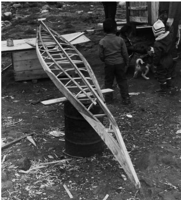
Figure 1.3 —Northwest Greenland kayak framework, Qaanaaq. The gunwales are constructed of several pieces of wood scarfed together. © Jens Ostergaard, 1995.
