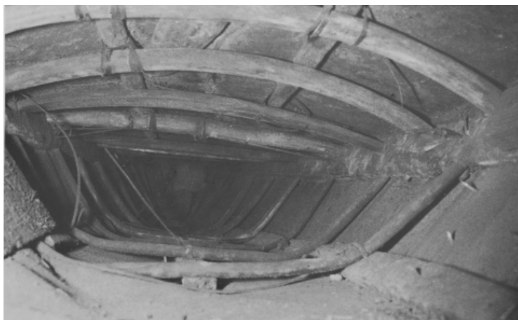
Figure 1.6b —Forward interior of the Lübeck kayak.
