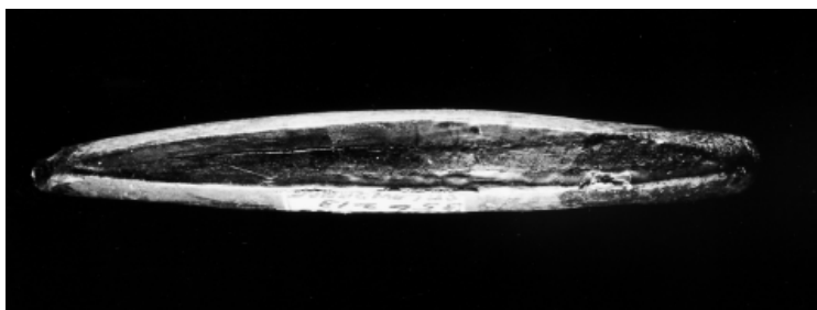
Figure 8.13c —View of Late Puvuk model showing flat bottom with hard chines. Photographer Vernon Doucette.
