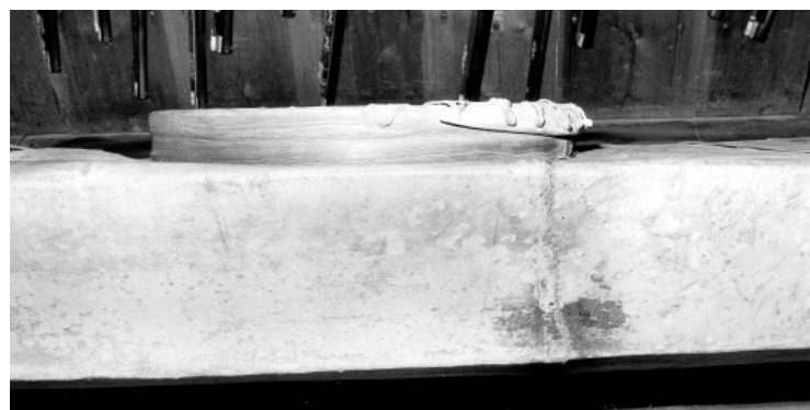
Figure 4.2 —Coaming of the Skokloster Palace kayak; port profile showing concave section forward and added lip aft for tuilik .
