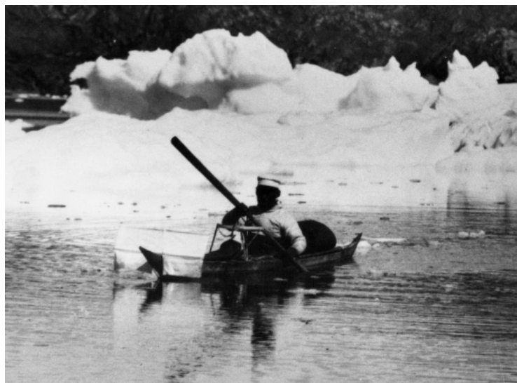
Figure 1.8 —Kayak with white cloth shooting screen and tray for the harpoon line, Uummanaq, West Greenland, c. 1900. Photographer Alfred Berthelsen, no. AI4067. Courtesy Danish Arctic Institute, Copenhagen.
