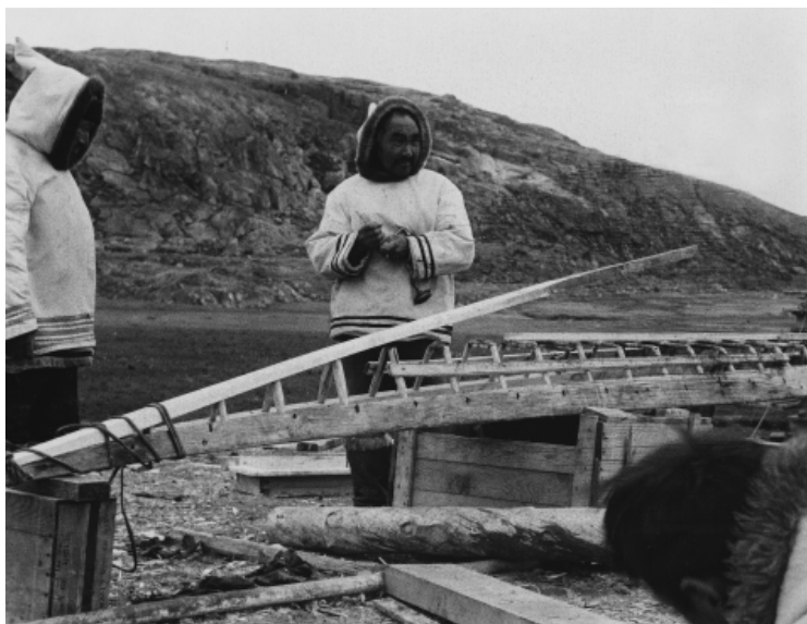
Figure 8.7 —Ainalik (right), assisted by Iyauituaq, installs a new niutaq , or cutwater strip, which will be bent down to meet the kuuyyaq , or keel, in a scarf joint. Photographer E. Arima, 1960. © Canadian Museum of Civilization, no. J16409.
